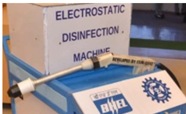
Electrostatic disinfectant spray machine for sanitising indoor areas.
