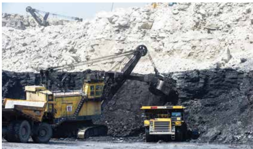
Shovel loading coal in the dumper.
